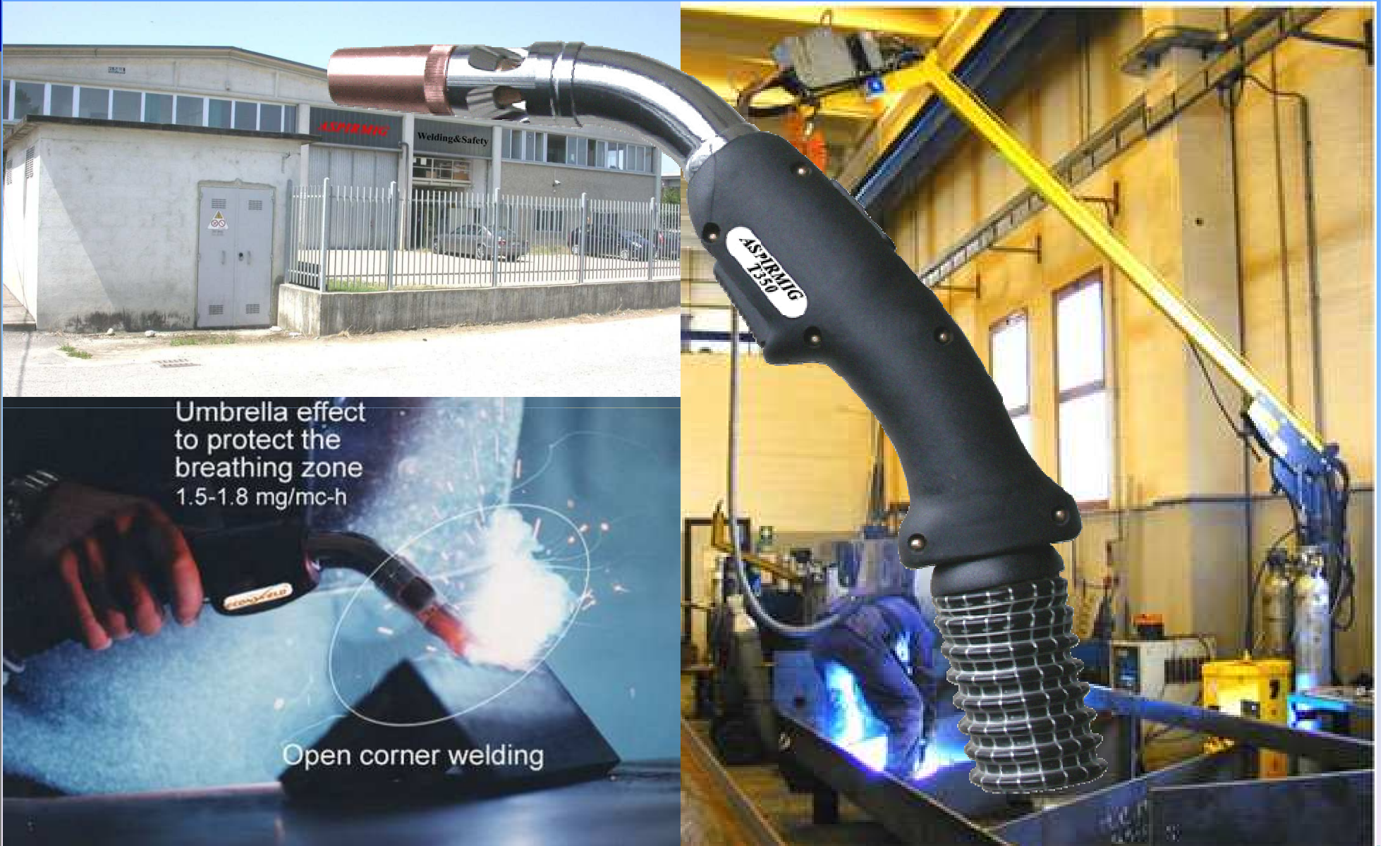
Econweld Project: research and testing fume capture efficiency of GMAW aspiring torch.
