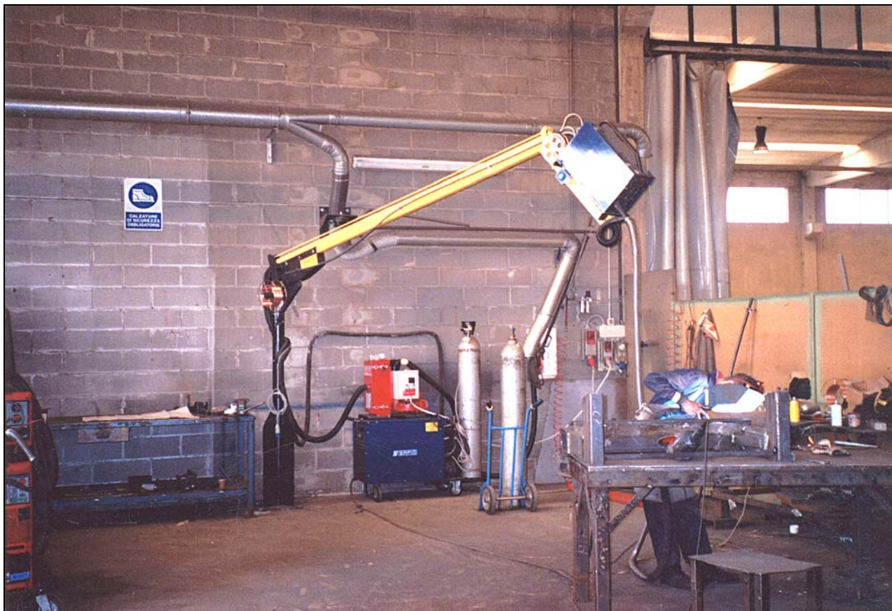
Comparison between the unused traditional suction system and the ergonomic system ASPIRMIG
