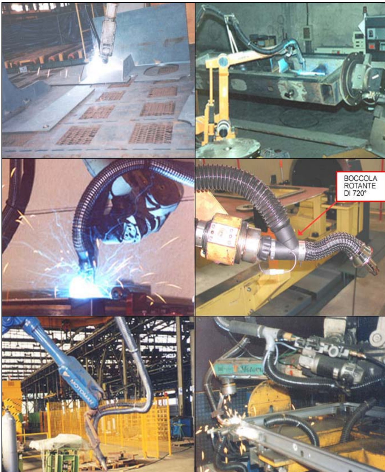
Some examples, of the easy installation of the torch with integrated suction of fumes on robotized welding processes of different brands: Motomann, Igm, Fanuc, Asea.
