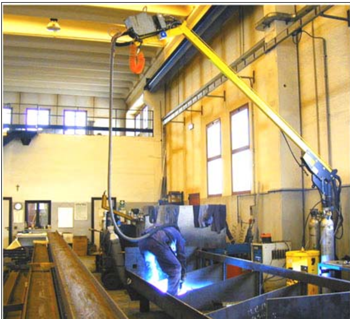
Suction of fumes before the breathing zone in all the workstations in accordance with HYGIENE, SECURITY and ERGONOMICS norms.
